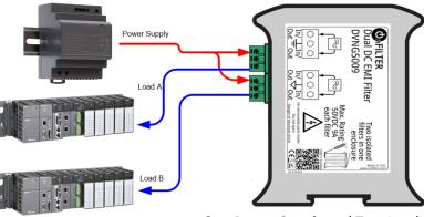
One Power Supply and Two Loads That Need to be EMI-Separated
