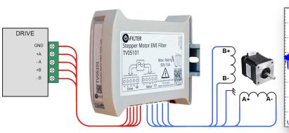
For maximum performance make sure that ground connection from the drive to the motor goes through the filter
