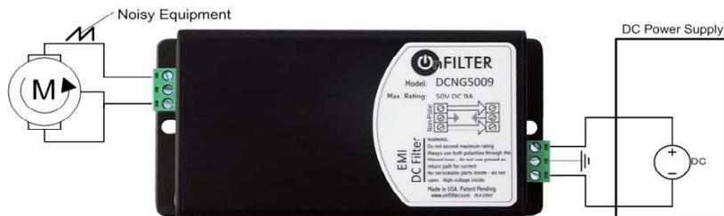
Figure 4. Filter Connection With Noisy Load and One Line Running Through Ground
