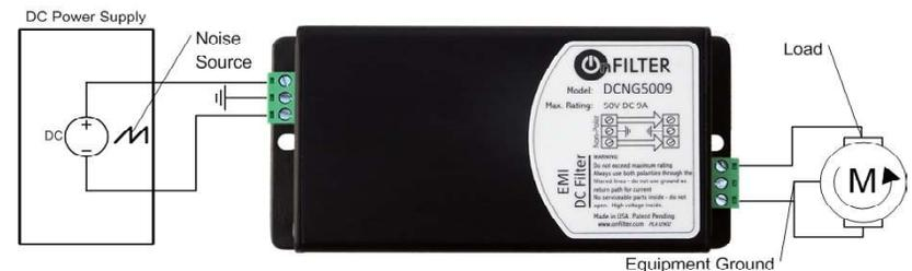
Figure 2. Filter Connection With Noisy Power Source and One Line Running Through Ground
