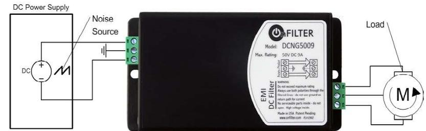
Figure 1. Filter Connection With Noisy Power Source
