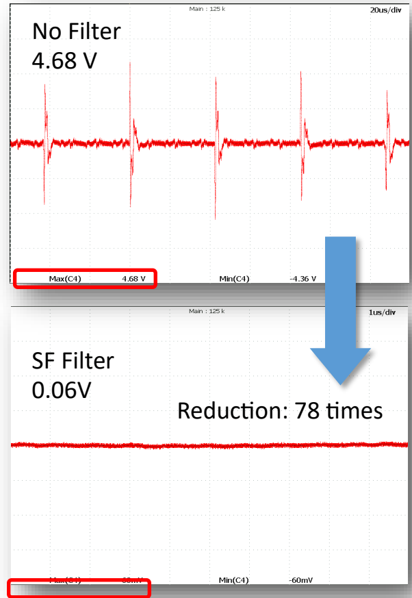
Current is measured with Tektronix CT1 probe 5mA/mV
